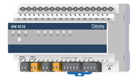
GW-EC10 is one of the smart lighting controllers in the GW series which is widely used in the electromechanical equipment control field of the intelligent lighting system. It is equipped with the functions of 1 Pyxos bus channel (abbreviated as PBUS), 2 RS485 channels, 1 RS485/RS232 channel, and 8 channels for digital input with optical isolation. The digital input can receive signals of switches, alarm devices, and infrared sensors, etc.
